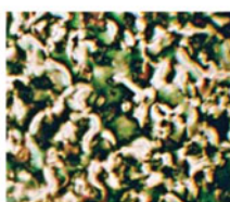
c). Schlieren texture of SmC phase (250X).
